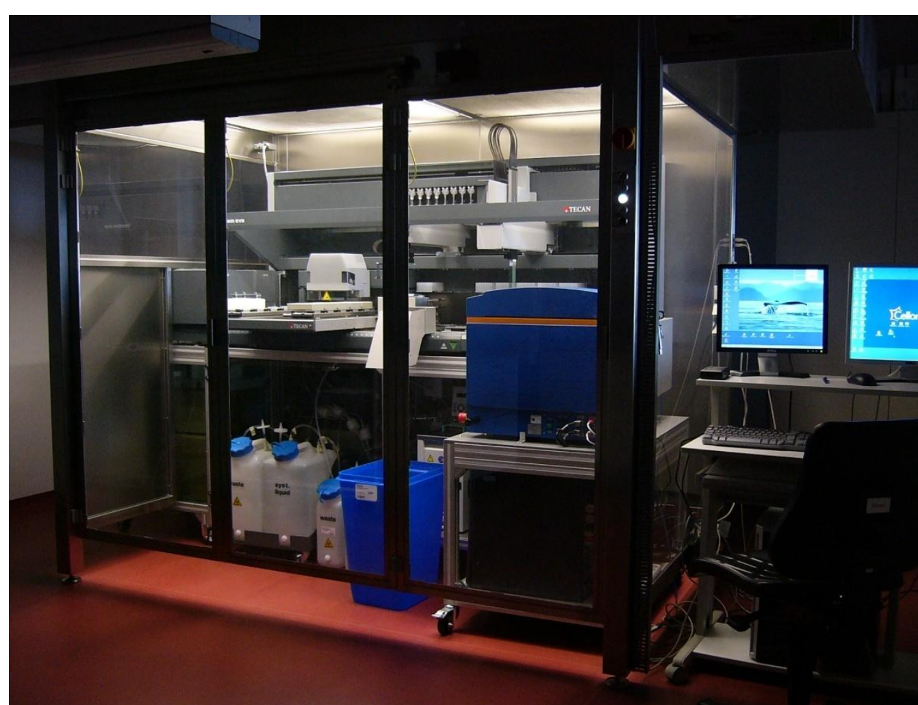
Fig.6: By means of a Tecan robot workstation aliquots of 40000 compounds are automatically added to the assay samples provided as aq. buffers in 113 x 384 well plates.
